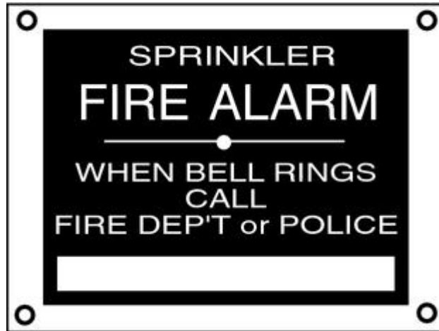
FIGURE A.8.17.1 Identification Sign.
